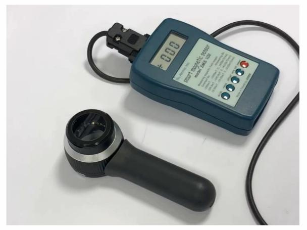
The invention provides a dermatoscope cap which enables shielding of the magnetic field, thus ensuring reduction of the magnetic induction of a dermatoscope.
